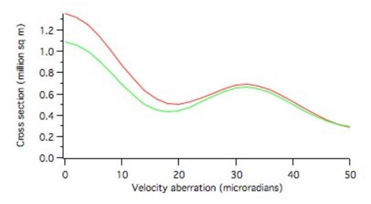
There is a 4 percent change in cross section at 32 microradians. This shows the extraordinay effectivenss of using small cubes with a floating mount to virtually eliminate the effect of thermal gradients.
