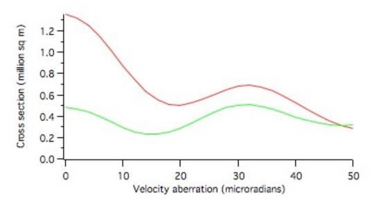
There is a 36 percent change in cross section at 32 microradians. This will eliminate the advantage of using the smaller cubes in terms of reducing thermal gradients.
